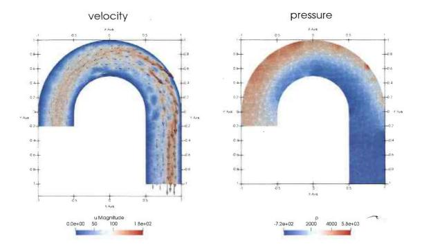
(c) 3 The following plots show the solution at one time step of the solution computed for a pulsatile boundary condition at the inlet  $\mathbf{u} = \sin(\omega t)\mathbf{g}(x)$ . The solution is shown at the time close before  $\omega t = \pi$ , i.e., after the maximum velocity.
